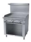
**Griddle Tops** - A 5/8" thick steel gnddle plate available with hi-low valve or super accurate thermostatic controls is an option (one per 12" section). A large 23" working depth with 18,000 BTU cast-iron H-style burner per 12" width of gnddle. High splash guards and a 4 ½" wide trough aid in grease control. Grooved gnddles are also available
