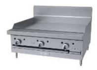
Griddle Tops - A 36" wide, 5/8" thick steel griddle plate available with hi-low valve or super accurate thermostatic controls is an option (one per 12" section). A large 23" working depth with 18,000 BTU cast-iron H-style burner per 12" width of griddle. High splash guards and a 4 ½" wide trough aid in grease control. Grooved griddles are also available.
