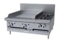
Griddle Top - A 24" wide, 5/8" thick steel griddle plate available with hi-low valve or super accurate thermostatic controls is an option (one per 12" section). A large 23" working depth with 18,000 BTU cast-iron H-style burner per 12" width of griddle. High splash guards and a 41/2" wide trough aid in grease control. Grooved griddles are also available.
