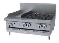
Griddle Top - A 12" wide, 5/8" thick steel griddle plate svailable with hi-low valve or super accurate thermostatic controls is an option (one per 12" section). A large 23" working depth with 18,000 BTU cast-iron H-style burner per 12" width of griddle. High splash guards and a 4 ½" wide trough aid in grease control. Grooved griddles are also available.
