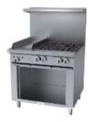
Griddle Top - A 12" wide, 5/8" thick steel griddle plate available with h-low valve or super accurate thermostatic controls is an option (one per 12" section). A large 23" working depth with 18,000 BTU cast-iron H-style burner per 12" width of griddle. High splash guards and a 4 ½" wide trough aid in grease control. Grooved griddles are also available.
